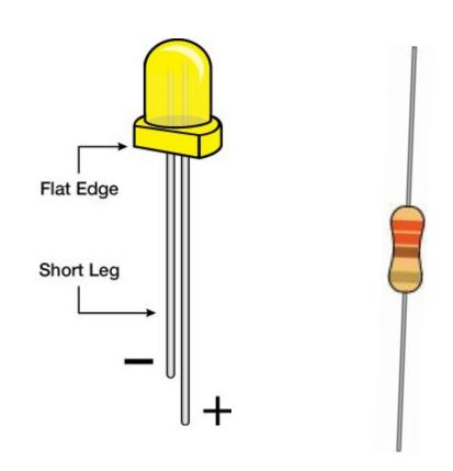
Tip: If a component is symmetrical, then it is probably omnidirectional. If there are asymmetric markings or geometry, then it might be directional.
